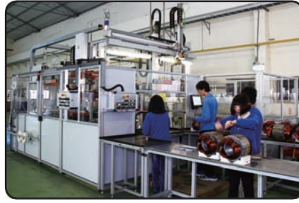
IE3全自動馬達繞線/ 入線/整形機與生產線 IE3 Automatic motor Stator winding/ Wedge Inserter/ Coil Forming Machinery and Production Line
